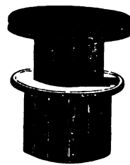
Fitting of Analyzing Prism upon the Eye-piece.
